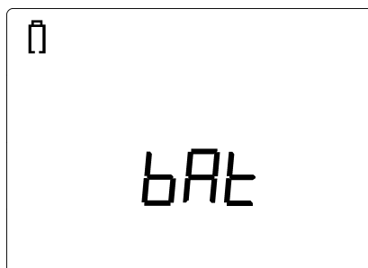
Figure 2.1: Discharged battery indication
